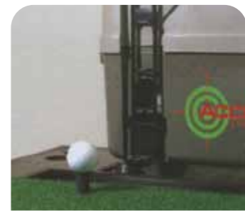
3 The dispenser tail will return to it is original position, right after a ball is placed on the tee.
