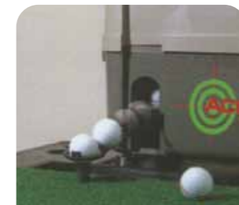
2 One ball will roll through the dispenser rail, and land on the tee.
